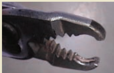
Open band pliers needed to close "open" bands securely. Your breeder or avian veterinarian clinic should be able to assist you with this procedure. These are expensive tools to purchase and technical skills are required to perform this operation.
