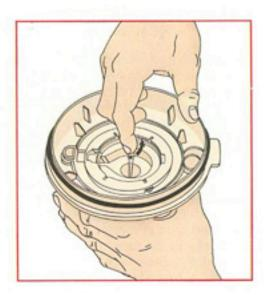
Replace impeller. Place the rubber shaft mount closest to plastic impeller fan into the impeller cover. Slide impeller into well, position cover and turn cover until it is secure.
