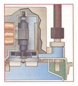
The impeller should be cleaned during every filter change. Twist cover until it comes free, and withdraw impeller with cover. Dirt and slime should be rinsed from the impeller before replacing. Be sure that all parts on the impeller shaft are not lost during cleaning.
