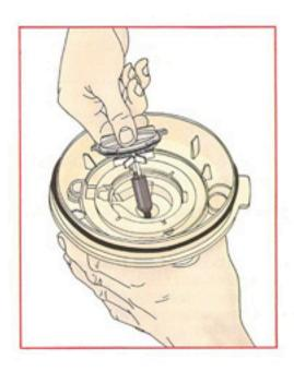
Occasional removal of the plastic well insert to ensure free water movement is recommended. To remove, press finger against insert to filter case and pull upward until insert is free, See Diagram.
